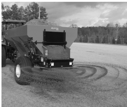
The Model 3500 spreading wet sand 480 inches wide in a smooth, even pattern.
